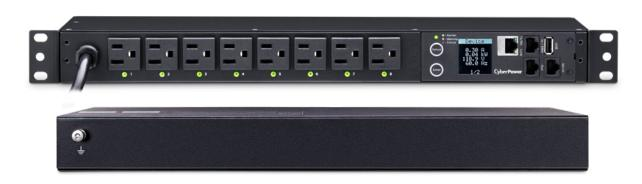
CyberPower Switched PDUs provide network-grade power distribution, remote/local monitoring, and outlet control to switch each outlet (device) on or off individually or collectively. Power status and PDU vitals can be monitored over the network, using the CyberPower Management Console and the RJ45 Ethernet port, or locally by using the digital LCD meter. Also, planned power cycling of attached equipment can occur without disrupting performance.
